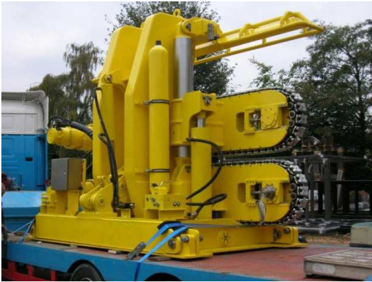
Typical 2 Track Tensioner with fixed height bottom track. Tensioners can be provided with horizontal or vertical tracks as shown above.
