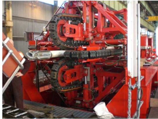
Typical 4 Track 40Te Tensioner mounted in a lay ramp. Tensioner is shown with test pipe for load testing.
