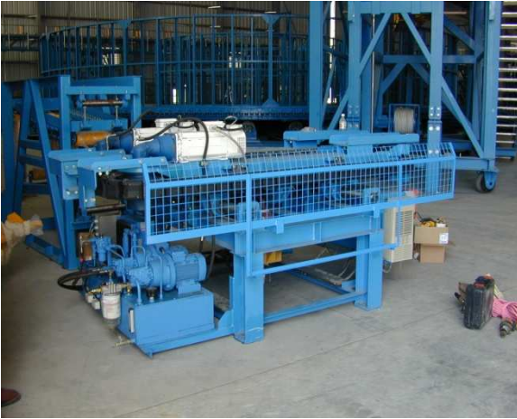
3 Tonne - 2 Track Tensioner used in the manufacturing process of tube umbilicals
