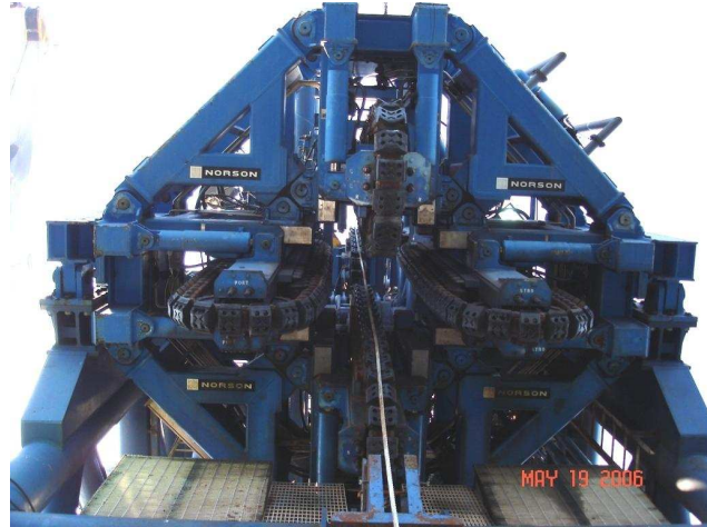
120 Tonne - 4 Track Tensioner used in the laying of offshore rigid or flexible pipelines
