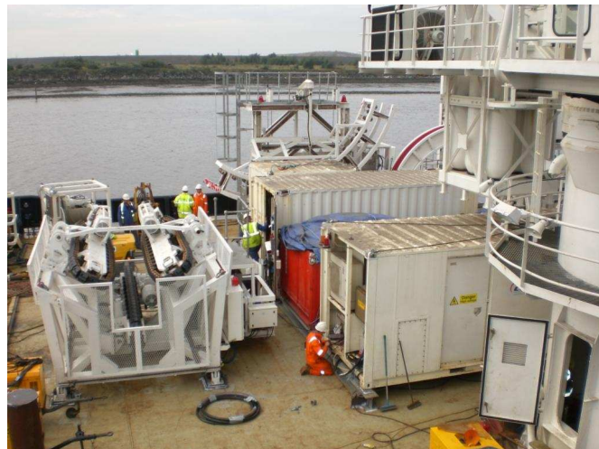
20Te Deck Mounted 3 Track Tensioner
