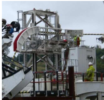
Simple spooling tower with inlet and outlet guide chutes
