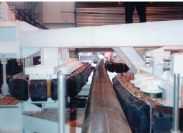
In-house Straightener trials on a 12"NB x 25mm wall X80 pipe.
