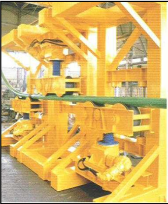
Modular Pipe Straightener that can be used with over or under wound pipe.
