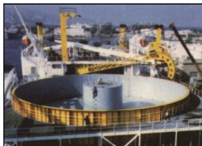
Tube umbilical being transferred from the manufacturing process into the storage carousel via the loading arm.
