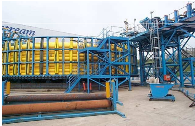
1500Te Flexible Pipe Carousel – Newcastle, England
