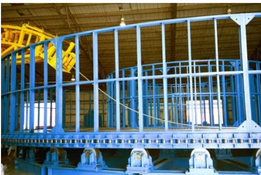
Tube umbilical being transferred from the manufacturing process into the storage carousel via the loading arm.
