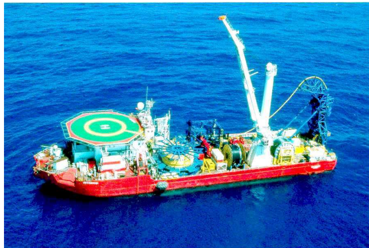
120Te capacity ramp with 1750Te horizontal reel
