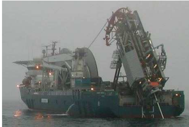
205Te capacity ramp with 2500Te vertical reel
