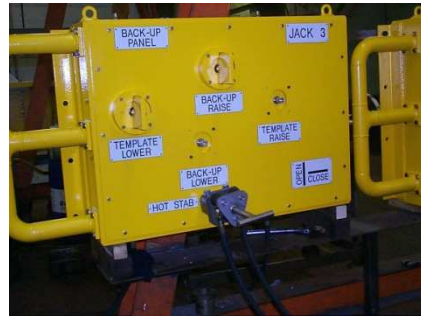
Typical ROV Panel and Jacking Cylinder used within the levelling system
