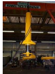
Typical ROV Panel and Jacking Cylinder used within the levelling system
